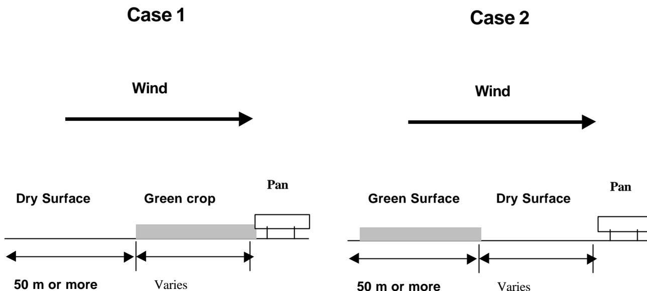
**Fig. 2.1: Definition sketch for computing pan coefficient**
